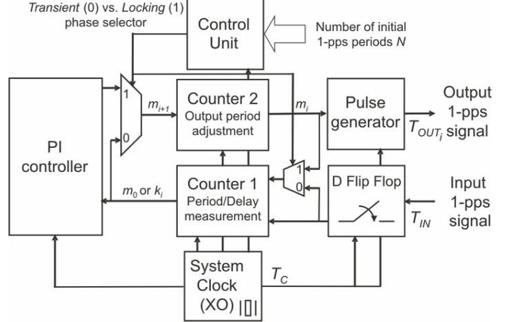
Fig. 2 – Architecture of the proposed synchronization circuit.
