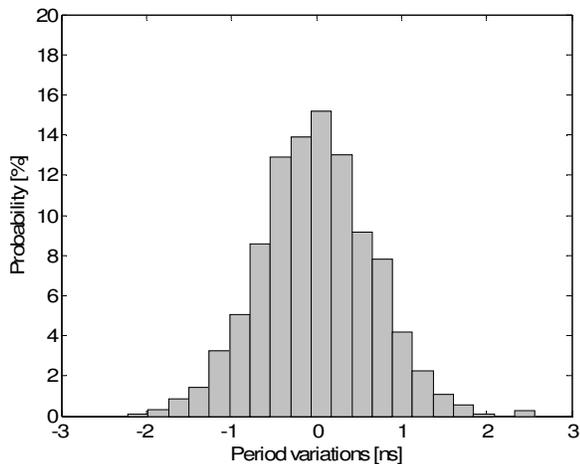
Fig. 4 – Histogram of the random jitter affecting two high-accuracy TCVCXO-disciplined GPS receivers Tekelec Epsilon Board II, after compensating the systematic trend.
