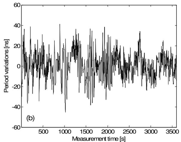
Fig. 5 – Time differences between the rising edges of a high-accuracy 1-pps signal generated by a Tekelec Epsilon board II used as a time reference and the rising edges of a less accurate Ublox Antaris 4 LEA-4T GPS module before (a) and after (b) applying the synchronization circuit.
