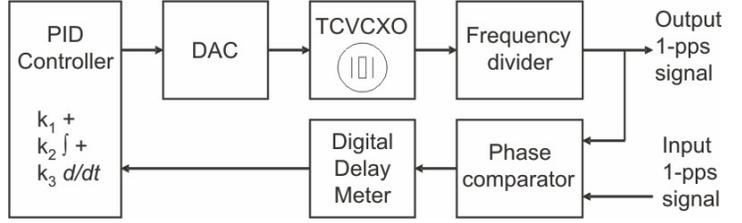
Fig. 1 – A typical high-accuracy GPS synchronization circuit based on disciplined VCXO technology.
