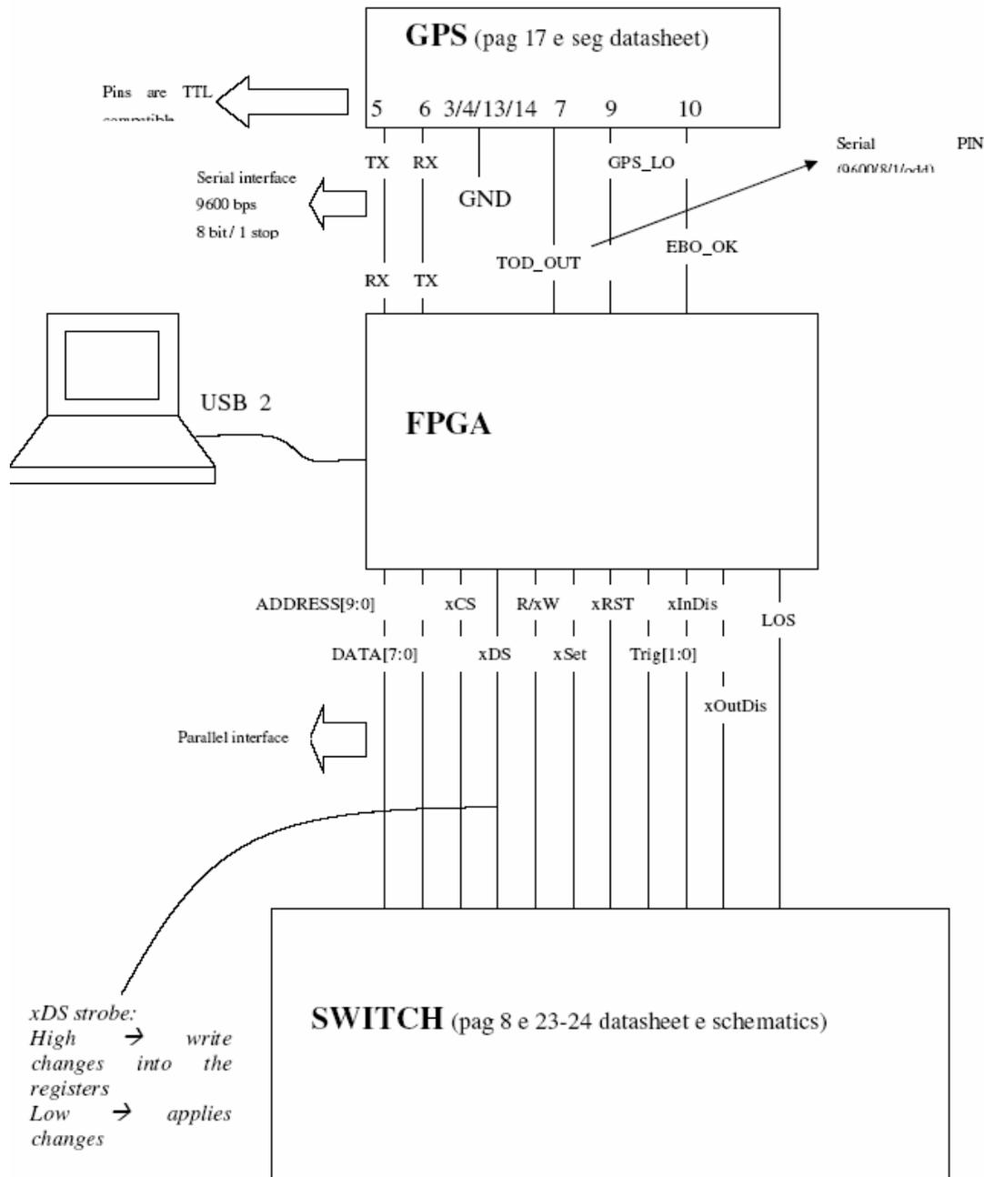
Figure 8. Switch Controller Block Diagram
