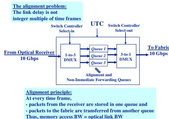
Figure 27. Architecture of electrical alignment
