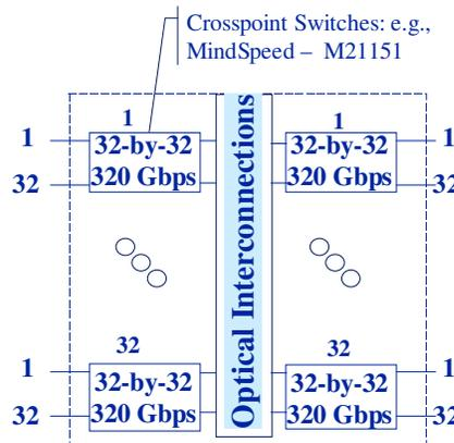
Figure 24. 10Tb/s switching fabric
