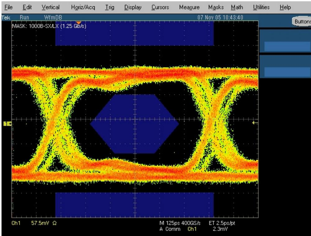
Figure 19. Eye Pattern with Mask: 1000B – SX/LX (1.25Gb/s) at location 4
