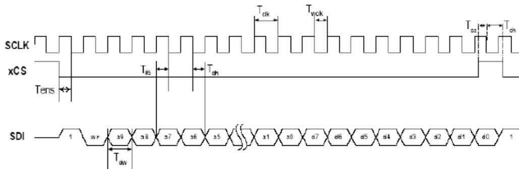
Figure 9. Timing Diagram for Writing
