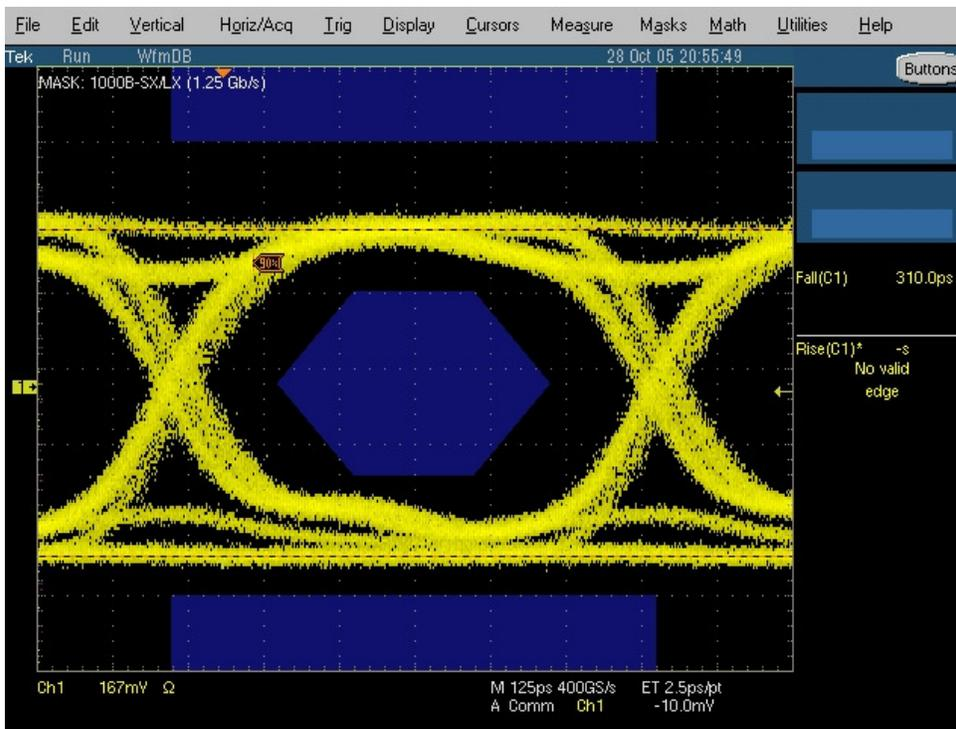
Figure 14. Eye Pattern with Mask: 1000B – SX/LX (1.25Gb/s) at location 1
