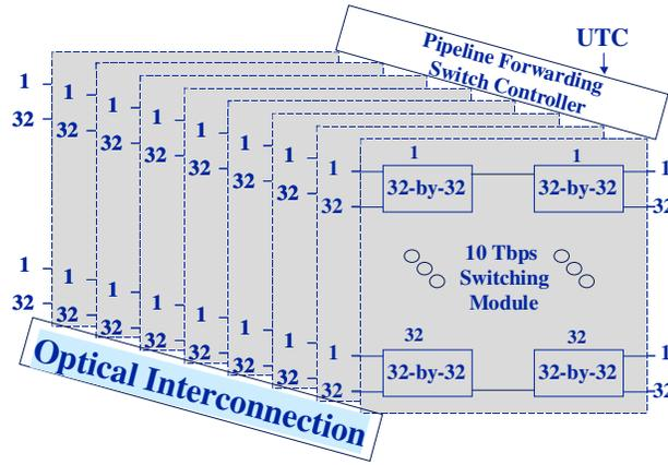
Figure 25. 40Tb/s switching fabric
