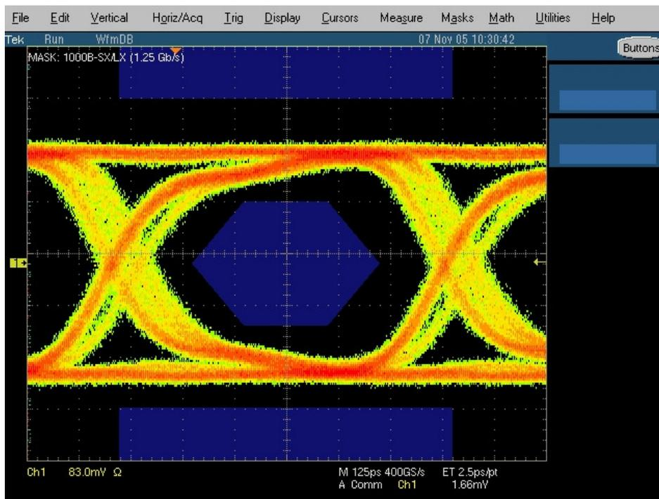
Figure 18. Eye Pattern with Mask: 1000B – SX/LX (1.25Gb/s) at location 3 with single mode Fibre
