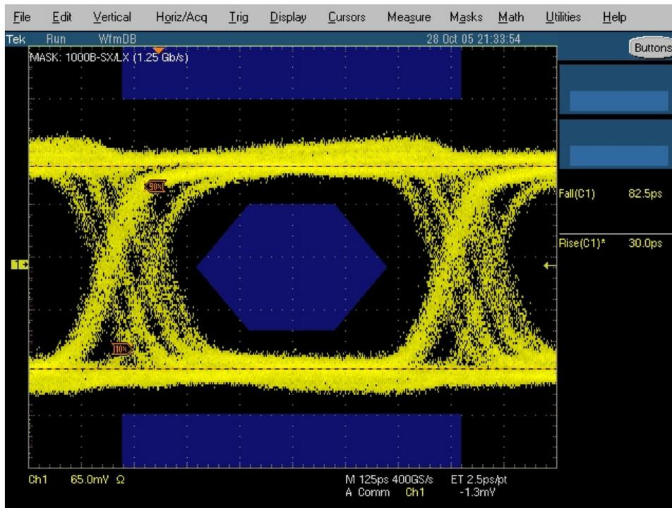
Figure 17. Eye Pattern with Mask: 1000B – SX/LX (1.25Gb/s) at location 4
