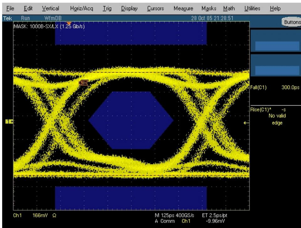
Figure 16. Eye Pattern with Mask: 1000B – SX/LX (1.25Gb/s) at location 3
