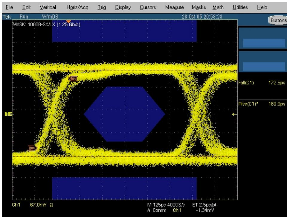
Figure 15. Eye Pattern with Mask: 1000B – SX/LX (1.25Gb/s) at location 2
