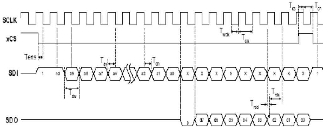
Figure 10. Timing Diagram for Reading
