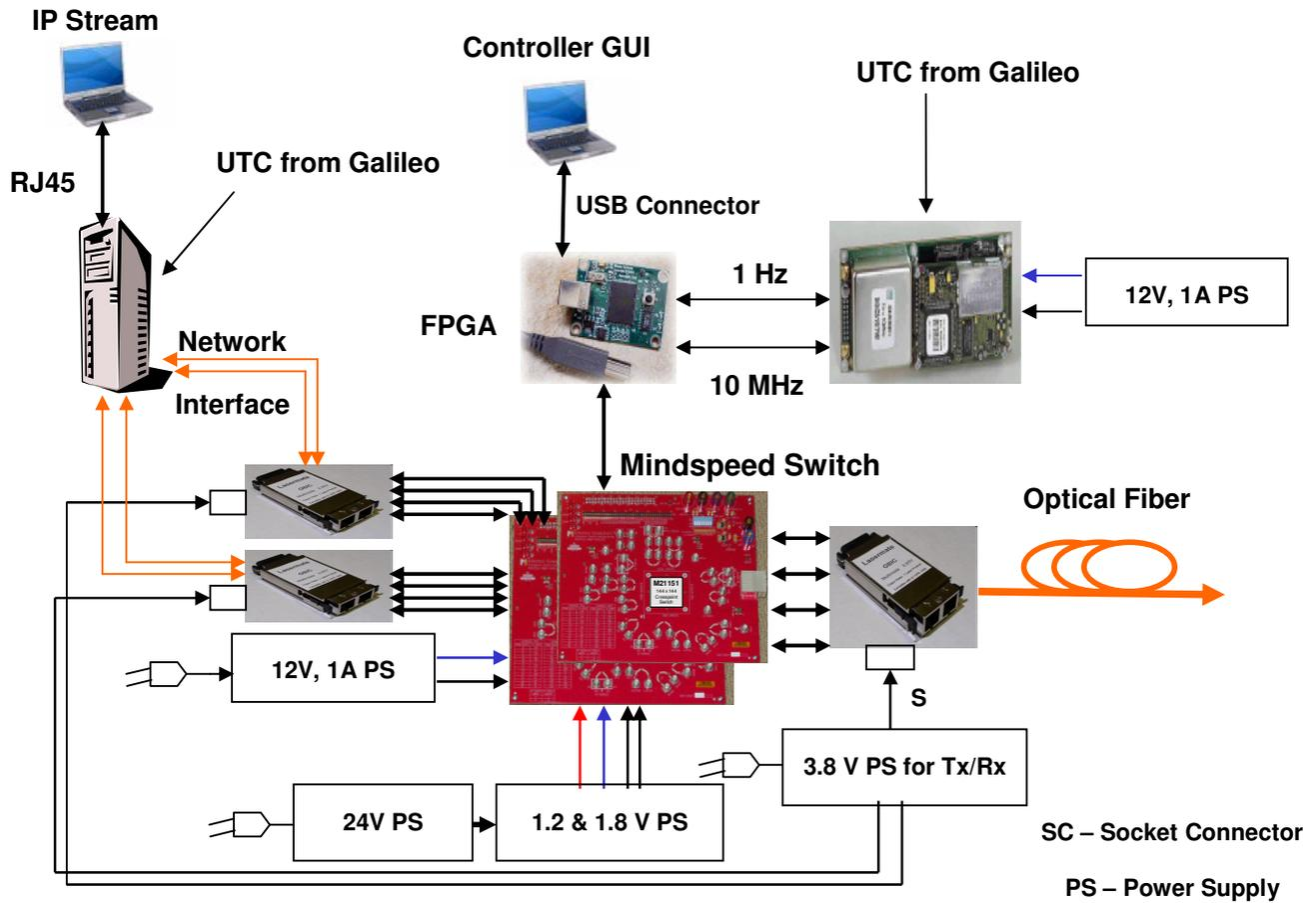
Figure 4. Detailed setup diagram
