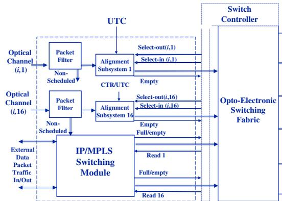
Figure 29. Hybrid IP/MPLS and TDS system
